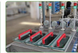
• Vacuum alarming for every section.
